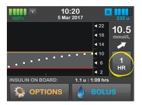
LOW shows when your most recent sensor glucose reading is less than 2.2 mmol/L.
