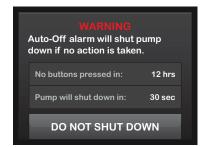
✓ The warning clears and the pump returns to normal operation.
