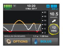
24 Hour Trend Graph shows you your current glucose reading along with the last 24 hours of sensor glucose readings.
