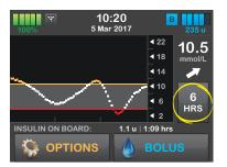
12 Hour Trend Graph shows you your current glucose reading along with the last 12 hours of sensor glucose readings.
