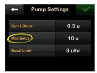
Using the on-screen keypad, enter the desired amount for maximum bolus (1–25 units) and tap
