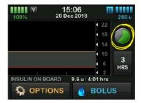
At the end of the 2-hour startup period, if you have not entered the sensor code, then you will be prompted to enter 2 calibration values. 2 blood drops will appear in the place where the countdown symbol was. If you entered a sensor code, the countdown symbol will be replaced with the current CGM reading.
