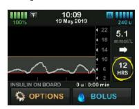
24 Hour Trend Graph shows you your current glucose reading along with the last 24 hours of sensor glucose readings.
