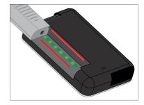
Push on the circular fill port next to the cartridge tubing to slide the cartridge onto the pump. Tap the UNLOCK icon when completed.
