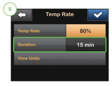
Tap Duration. Using the onscreen keypad enter desired length of time for Temp Rate. Тар 🗸 .
