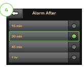
Select the button that corresponds with the time you would like the Resume Pump Alarm to display.
