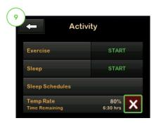
To stop Temp Rate at any time, tap Options > Activity and then press the X.
