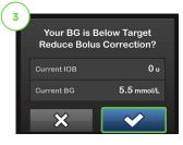
If a BG is entered that is below the target, but above or 3.9 mmol/L, you will be offered the option to reduce the bolus amount. To accept that reduction tap ; otherwise, tap x
