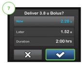
The delivery screen will confirm how much insulin will be delivered up front, how much will be delivered over time, and the delivery duration. Tap very to start the bolus.
